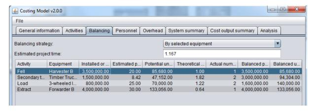
Now the Estimated project time cannot be adjusted and is set to accommodate the selected machine constraint. The number of other machines in the system is decided based on the estimated project time.\
